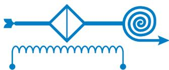
The gas sample is extracted through a double dust filtration and conditioned before transport, in order to have all moisture and condensable components removed prior to its analysis. With a dew point below  $-20^{\circ}\text{C}$  ( $<1000$  ppm  $\text{H}_2\text{O}$ ) the clean & dry sample is transferred to the analyzer via an unheated line.
