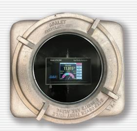
CAI has selected an ATEX/IECEx-rated NEMA7 explosion-proof housing to allow the GPA2000 to be installed in areas classified as hazardous. The threaded-lid cover has a see-through viewing window allowing for convenient viewing of the display to confirm operation of the unit at all times. By placing the GPA2000 into an EXD housing, CAI has eliminated the need of an X-Purge controller and the continuous delivery of an inert purge gas to meet the hazardous area installation requirements.
