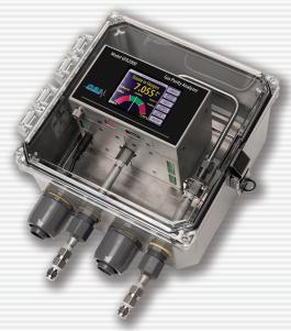
IP66/NEMA4X rated, UV and corrosion resistant polycarbonate enclosure. A clear hinged door allows viewing of the display and quick access to the instrument. The sealed enclosure protects the GPA2000 from dust, weather and hose-directed water. Liquid tight gas ports and flexible, non-metallic cable conduit ports are located on the bottom edge of the N4X wall mount enclosure.
