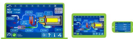
Adopt the no-screen version and avoid the pollution related to the screen manufacturing and recycling cycle. The analyzer is connected with your device (computer, tablet or smart-phone). Simultaneous multi-screen remote access via Wifi or Lan using the dedicated application ENVEA Connect™ for control, diagnostics, software update...
